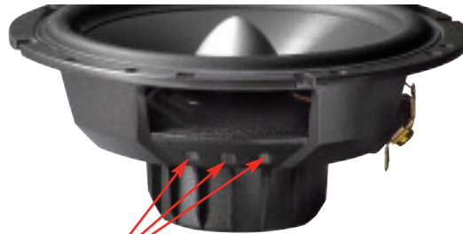
Figure F: Vent holes equalize air pressure on both sides of the spider for more linear cone travel.
